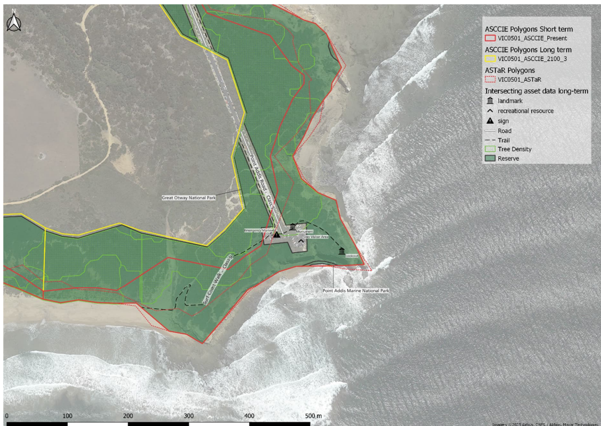
Figure 4.2: Example of asset data intersecting short-term and long-term ASCCIE and ASTaR polygons.
