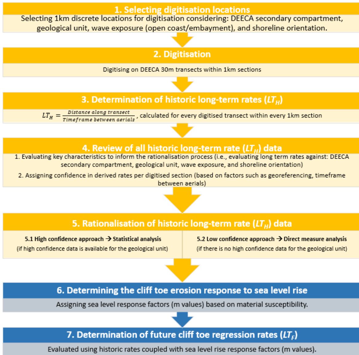
Figure 5.4: Process used to derive historic (yellow) and future (blue) cliff toe regression rates
