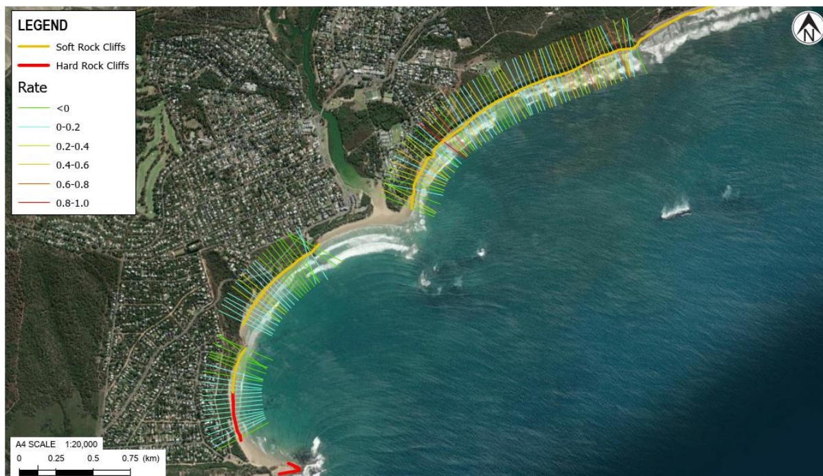
Figure 3.5: Anglesea rates from aerial imagery (dated between 1962-2020) within the VCMP database, where erosion rates are provided in m/year
