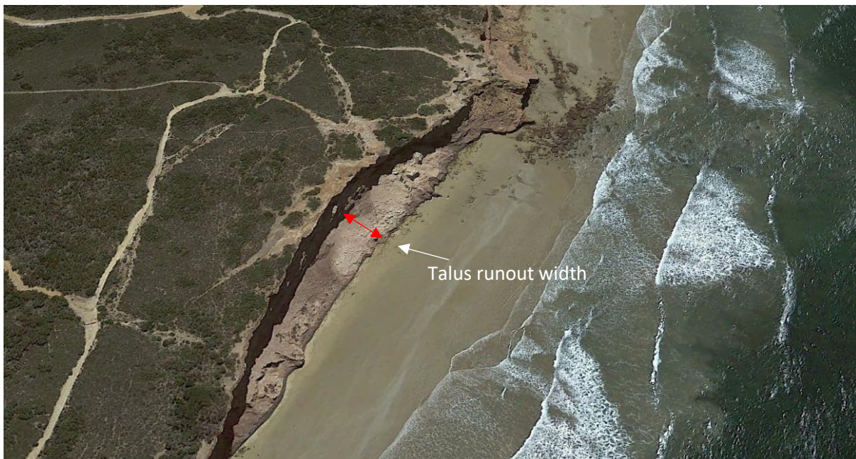
Figure 4.7: Talus runout at the base of a cliff east of Anglesea (source: Google Earth, 28/1/2019)
